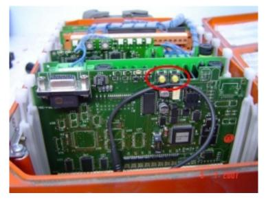
For model 730 (older versions): The buttons are located on the underside of the top PCB boards in the receiver. By undoing 2 brass screws at one end of the top PCB boards, the 2 boards will swivel up and the buttons can then be seen on the underside.
